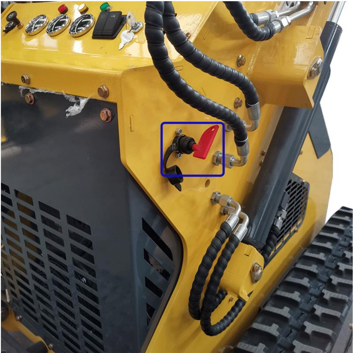
main power switch
